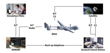
Figure 4 RPAS simulation architecture
