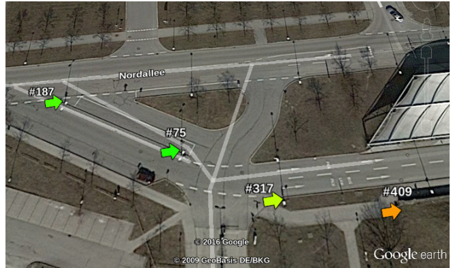
Figure 2: GCPs from the Munich airport test site (close-up)
