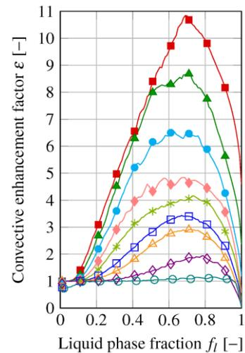
Figure 6: Convective enhancement factor over liquid phase fraction
