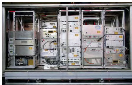
Fig. 2. Frontal view of the automated measurement container, 3.1 m wide, gross weight, 1450 kg.
