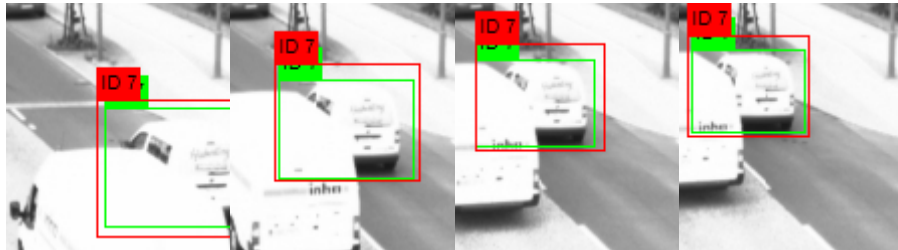
Figure 6: Results of occluded vehicle tracking (red) comparison with ground truth data (green).
