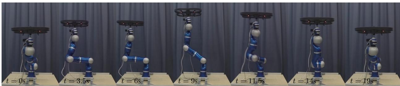
Fig. 7. Picture sequence from the experiment with the controller from Section III-C, the indicated time instants correspond to the plot in Fig. 10. A short video by the authors of this paper showing the VTOL UAV landing system demonstrator and some of the conducted experiments is provided online [18].
