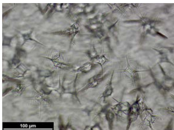
Figure 1: Optical microscope image of small crystallites in the glass, forming a spinifex texture.
