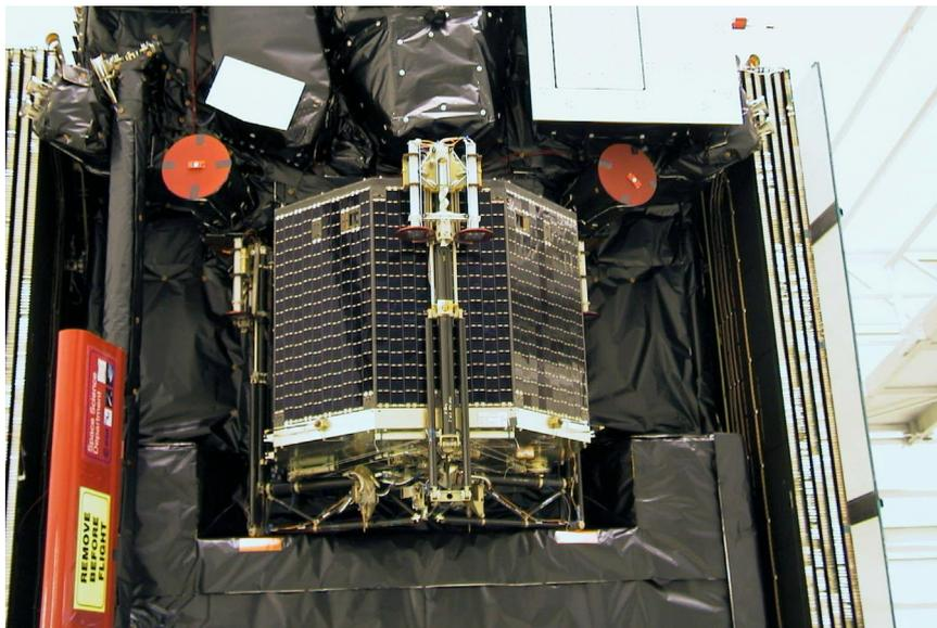
Fig. 2. Rosetta Lander as attached to the Orbiter [6].
