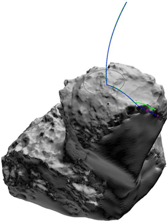
Fig. 4. Descent and bouncing trajectory of Philae [3].
