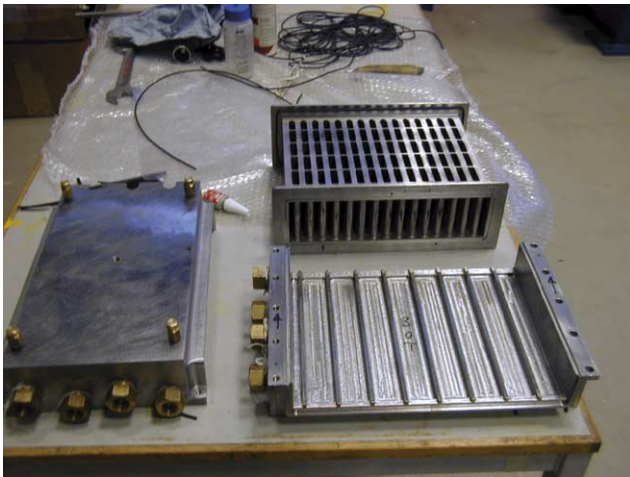
Fig. 7. One of the three heat exchanger stages belonging to the HES. Three such stages compose the HES. Horizontal ducts are for combustion exhaust products and vertical ducts are for water cooling.
