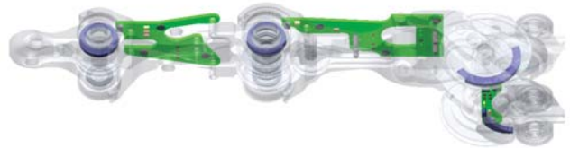
Fig. 11: Green: electronic board. Purple: magnets
