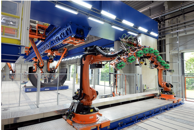
Fig. 2. Two industrial manipulator systems used at the Center for Lightweight Production Technology : a robotic portal system in the background (MFZ) and two robots on a linear axis (TEZ) in the foreground
