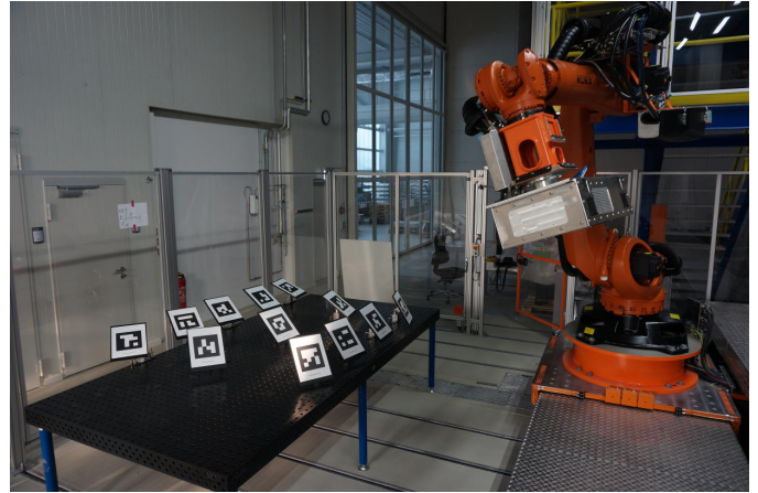
Fig. 3. The process environment, showing the AprilTags markers attached to a table on the left side and the industrial manipulator used (KUKA KR210) with the attached end effector described in section II-B
