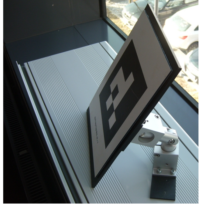
Fig. 5. The mounting of a marker, showing the AprilTag on the left and the adjustable attachment of the marker to the base on the right side
