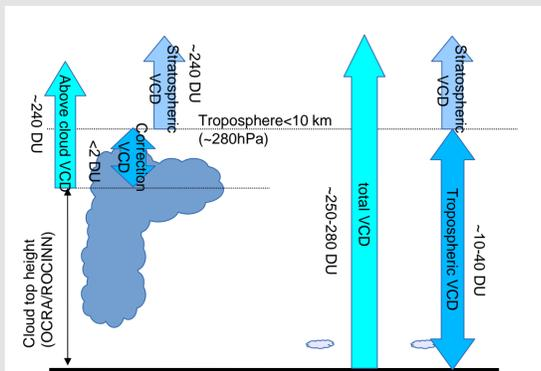
Fig 1: Principle of the convective cloud differential method to retrieve tropospheric ozone column.
