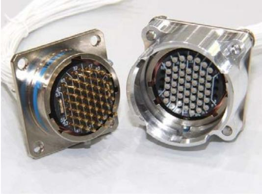
Fig. 7: Umbilical Connector (Flight Model)
