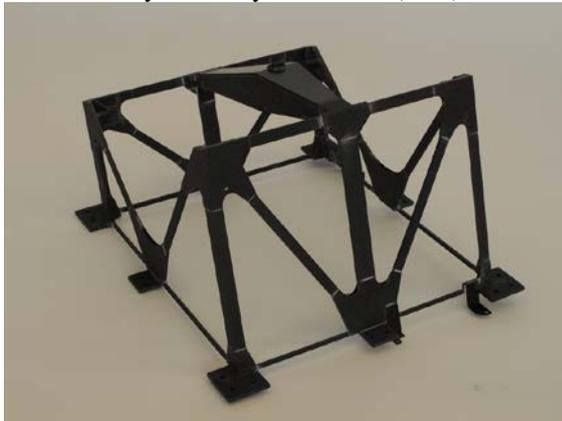
Fig. 5: MESS structure STM 2.2 (without MLI)<sup>4</sup>
