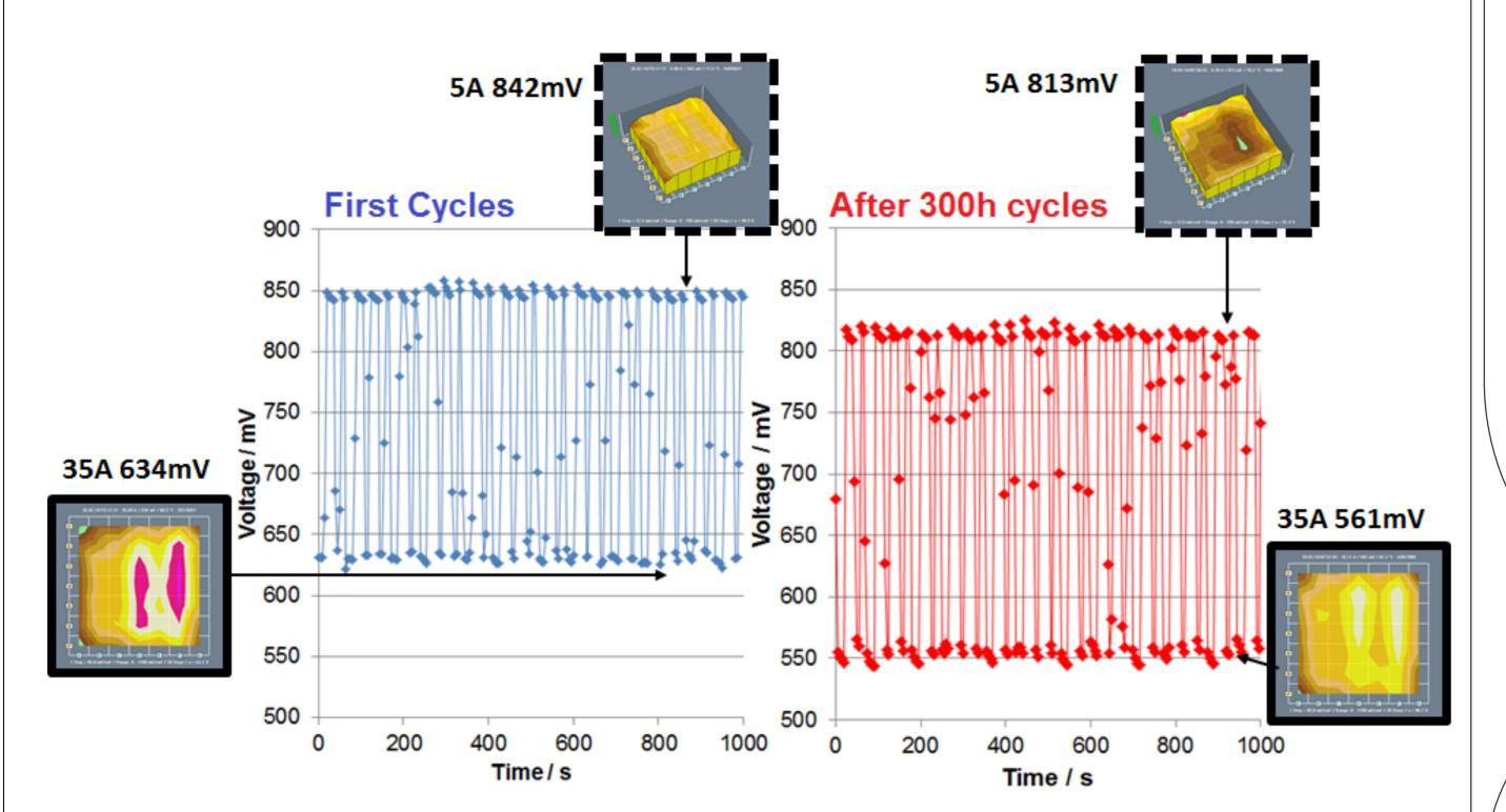
Degradation during the cycle@0.2 A/cm<sup>2</sup>: 100 μV/h Degradation during the cycle@1.4 A/cm<sup>2</sup>: 200 μV/h
