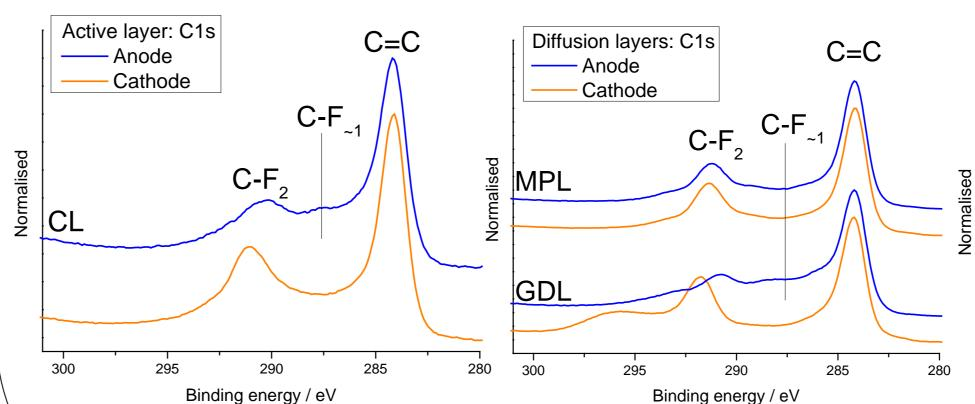
Partial defluorination of anode side ionomer (active layer) and PTFE (diffusion layers)
