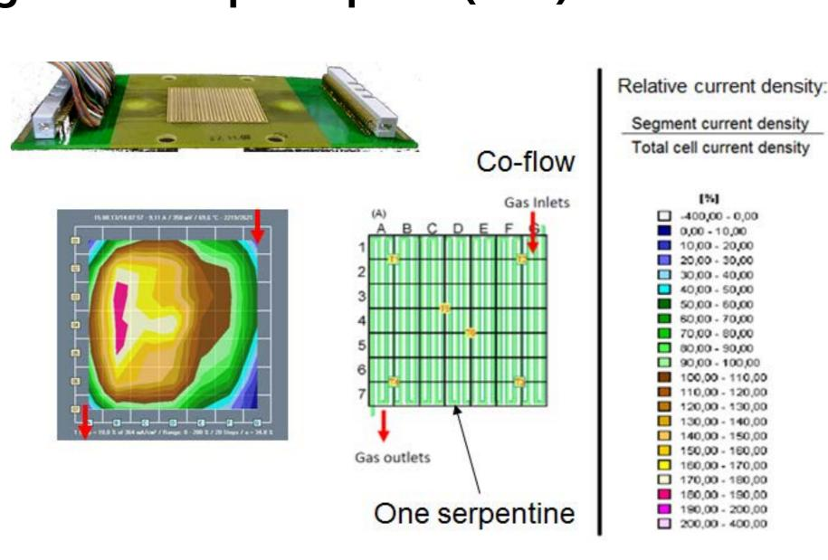
DLR segmented bipolar plate, based on printed circuit board (PCB) technology for current density distribution measurements
