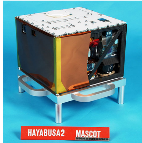
Figure 8L: MASCOT QM after passing successfully its Thermal Vacuum and Random Vibration test.
