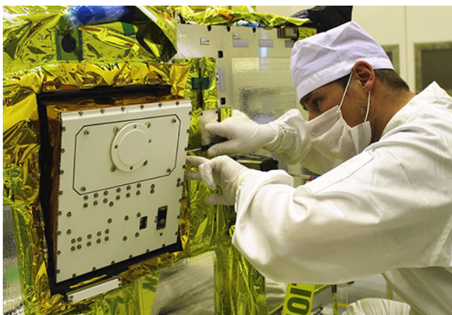
Figure 9L: MASCOT FM Final integration steps at Hayabusa2.
