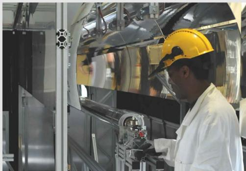
Figure 2: Linear focus solar simulator
