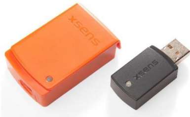
Fig. 2. MTw motion tracker (left) Awinda Dongle (right). The users carried the MTw and the Dongle was connected to a laptop to receive the data from the MTw.
