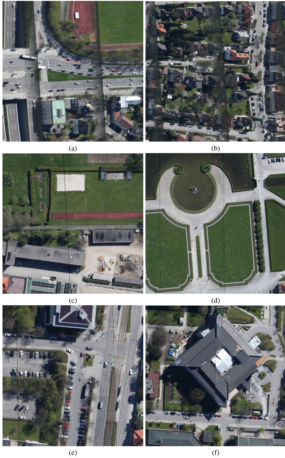
Fig. 5. Cropped part of the mosaic image showing the borders between two images. The images are stitched together without smoothing purposely to better show the accuracy. The black line shows the image border. The (a) and (b) show front camera images, while the rest are nadir images. The (f) shows the parallax on a taller building.
