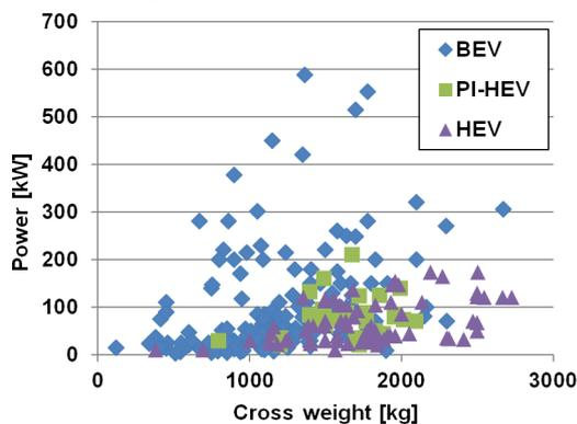
Figure 8: Installed maximum power of electric machine plotted against the vehicle cross weight per electrification concept
