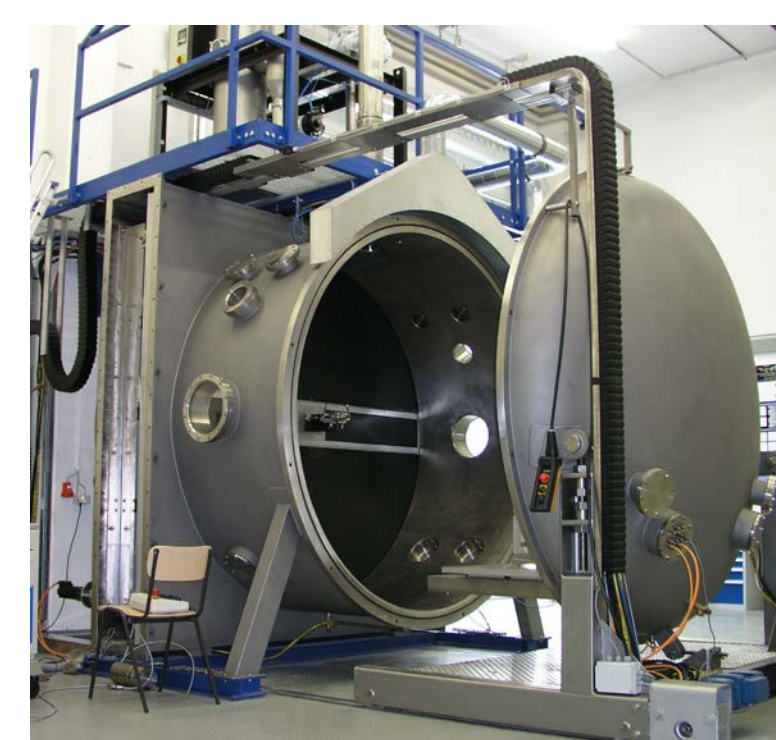
Vacuum plasma spraying chamber
