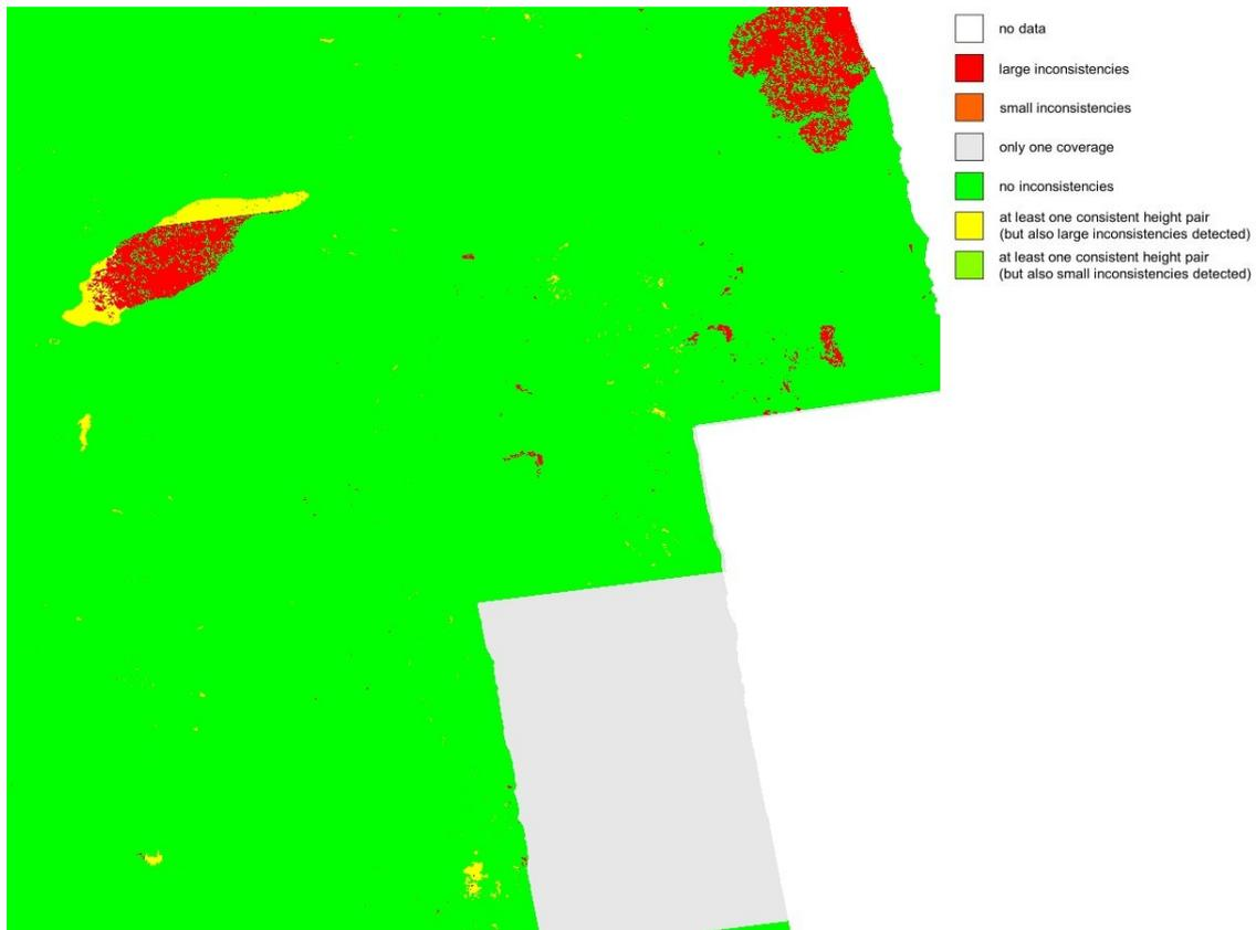
**Figure 10: Quicklook of the consistency mask with legend. In this example the yellow and red inconsistent height values are caused by water bodies.**
