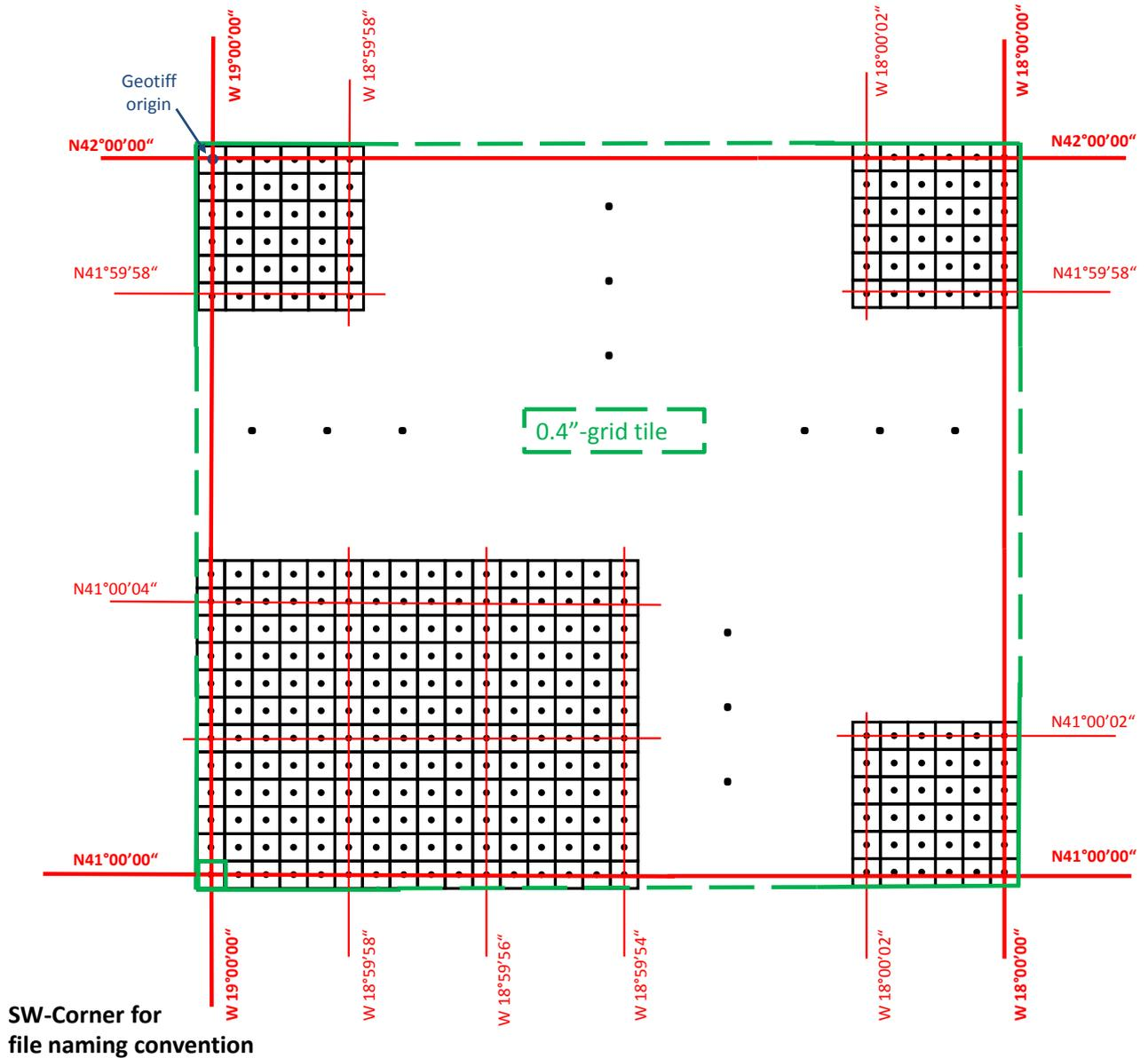
**Figure 1: Grid definition for DEM tiles. The bounding latitudes and longitudes (e.g. W 19°00'00", N41°00'00") are always integer values. The file naming convention refers to the southwest corner (SW), here N41W019. Please note that the GeoTIFF header refers to the pixel center in the northwest corner.**
