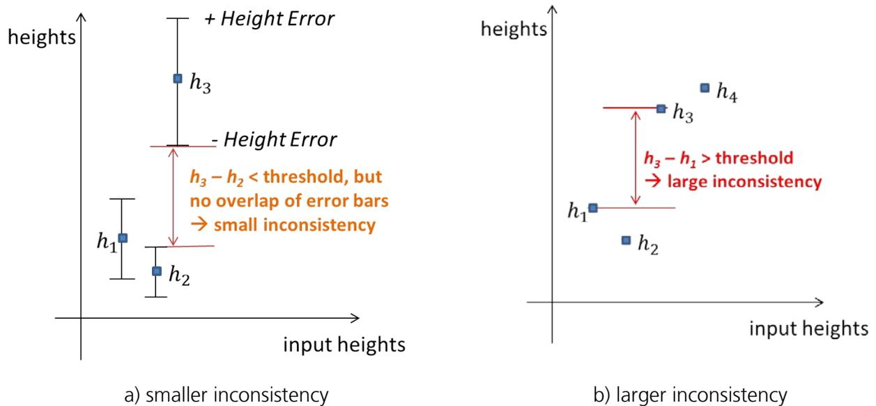
**Figure 9: Detection of a) smaller inconsistency between  $h_3$  and  $h_2$  because their error bars do not overlap and b) larger inconsistency between height groups  $(h_1, h_2)$  and  $(h_3, h_4)$ .**
