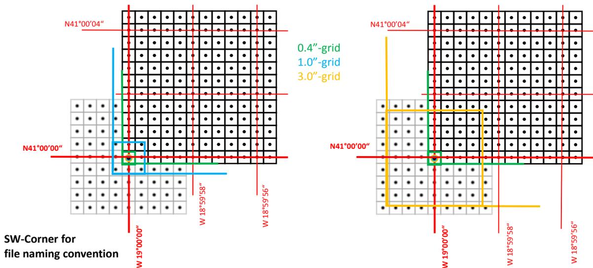
**Figure 15: Grid definition and pixel extent for DEM tiles with different pixel spacings: black grid/green square: original 0.4-arcsecond grid, blue square: one 1-arcsecond pixel; yellow square: one 3-arcsecond pixel.**
