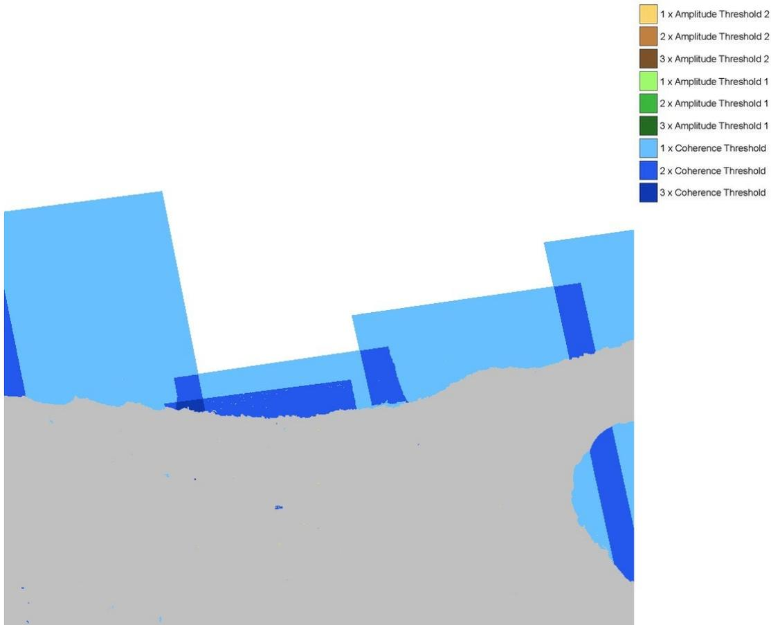
**Figure 5:** Quicklook of the water mask with legend, the color indicates the number of water detections. Note that if both coherence and amplitude methods detect water, the coherence counter will be displayed.
