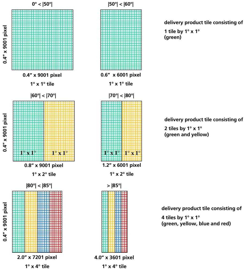
**Figure 13: Latitude dependent coverage of TanDEM-X DEM tiles.**
