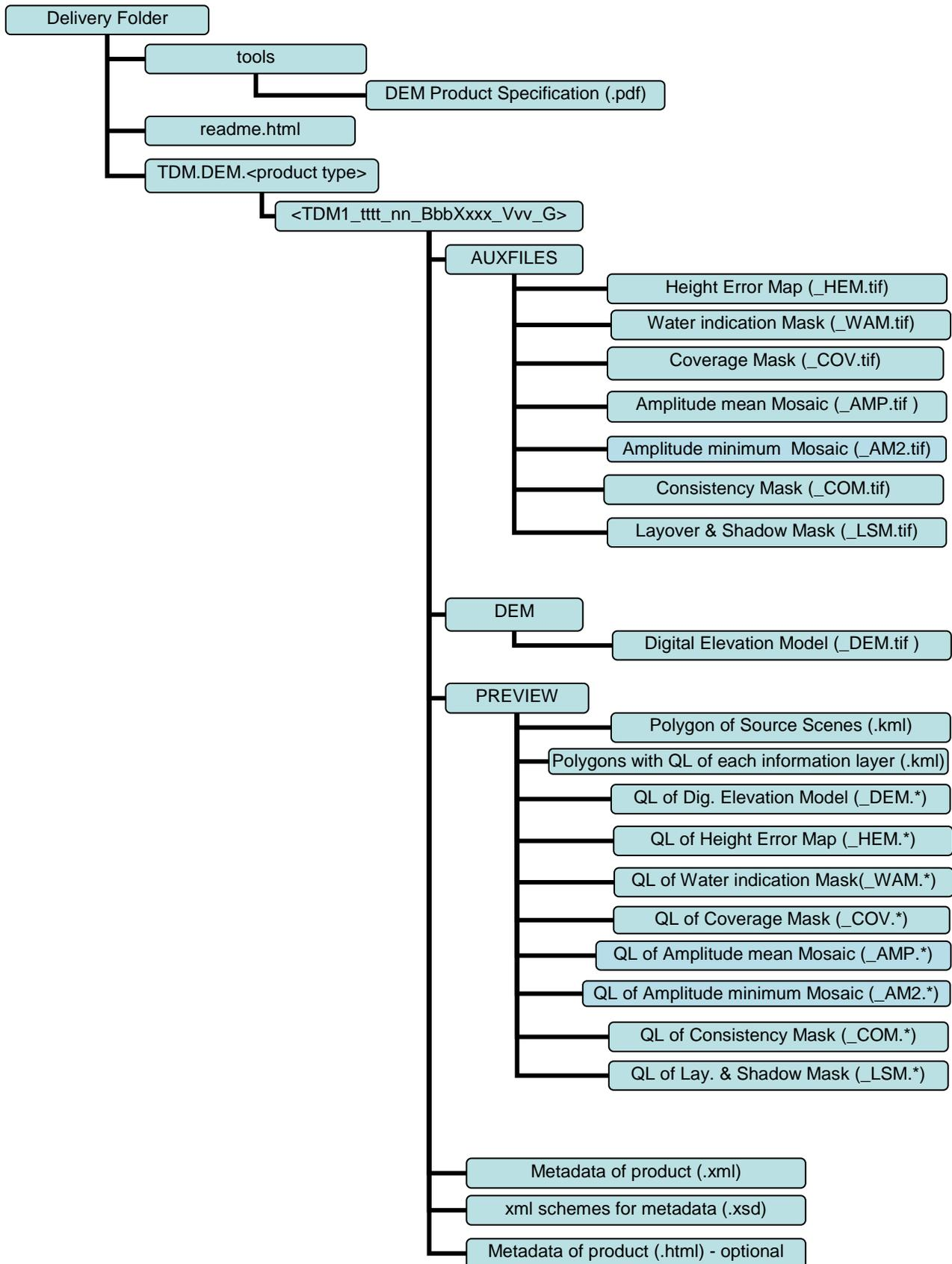
Figure 12: Directory structure of DEM delivery, add-on layers in grey, \* stands for PNG (png) or GeoTIFF (tif).
