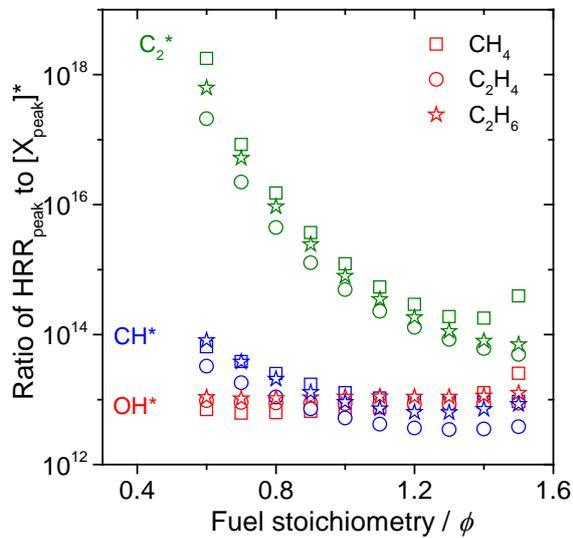
**Fig. 10:** Comparison of the ratio of heat release rate to ratio of peak concentration of chemiluminescent species ( $OH^*$ ,  $CH^*$ ,  $C_2^*$ ) at different fuel stoichiometry and for three different flames ( $CH_4$ -,  $C_2H_4$ -,  $C_2H_6$ -air). The calculations are performed for 298 K initial temperature and at atmospheric pressure.
