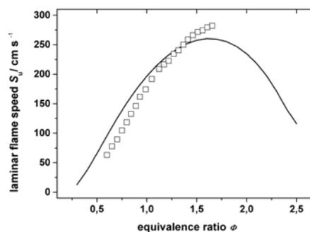
**Fig. 6:** Measured and calculated laminar flame speed for mixture I at ambient pressure and at preheat temperature of 473 K; oxidizer: synthetic air (80% N<sub>2</sub>, 20% O<sub>2</sub>). Solid line: simulations based on the mechanism of Li *et al.* [67]
