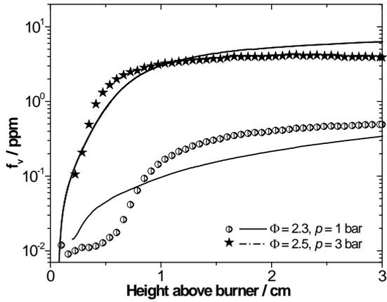
**Fig. 8:** Calculated and measured soot volume fractions  $f_v$  for the laminar atmospheric  $C_2H_4$ /air flame:  $p = 1$  bar,  $\varphi = 2.3$  and  $p = 3$  bar,  $\varphi = 2.5$ . Symbols – experimental data [72]; lines – calculations.
