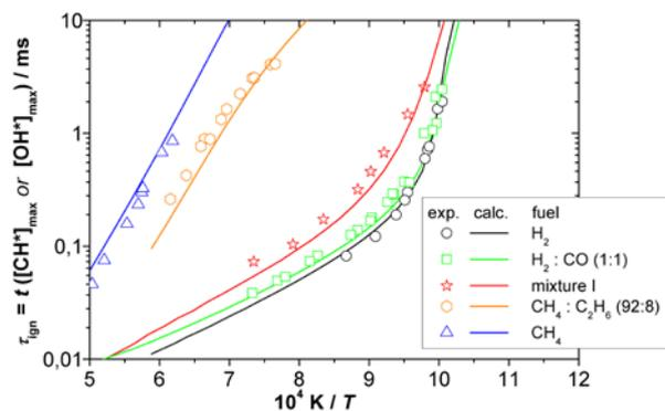
**Fig. 5:** Measured and calculated ignition delay times of different fuels at stoichiometric conditions and a pressure of 4 bar, diluted 1:5 in Argon; oxidizer: 79% Ar, 21% O<sub>2</sub>. Lines: simulations based on the mechanism of Li *et al.* [67]. Black: H<sub>2</sub> [65], green: 50 vol% H<sub>2</sub> / 50 vol% CO [68], red: mixture I, orange: reference gas (natural gas) [68], blue: CH<sub>4</sub> [69]
