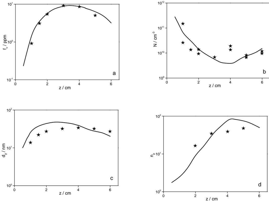
**Fig. 9:** Comparison of calculations [27] with experiments a) soot volume fraction, b) particle number density, c) average primary particle diameter, and d) average number of primary particles per aggregate. Measured data have been obtained in diffusion co-flow flames for a) [73], b) [74], c) [75],
