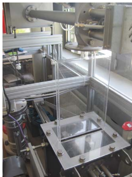
Figure 3 Test-bench with acryl glass reactor for moving bed reactor
