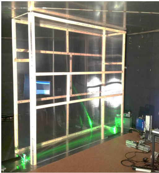
Fig. 2 PIV imaging setup for the investigation of RBC within a confined rectangular cell inside the Barrel of Ilmenau . Right: schematic of the global flow pattern within the RBC cell, PIV measurement setup and coordinate system
