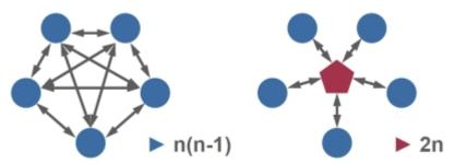
Figure 1: Interfaces in MDO Design Process without (left) and with (right) CPACS<sup>5</sup>
