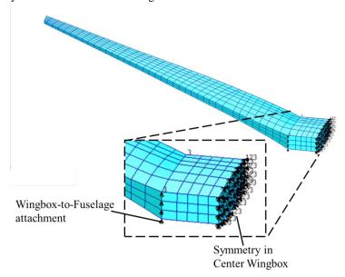
Figure 3: Boundary Conditions of Wingbox
