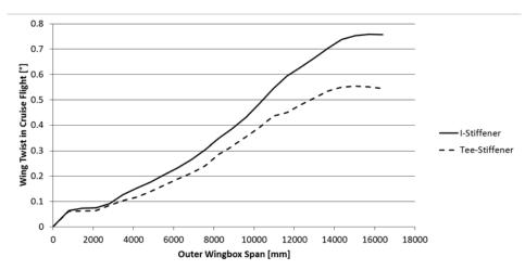
Figure 10: Comparison of Wing Twist in Cruise Flight
