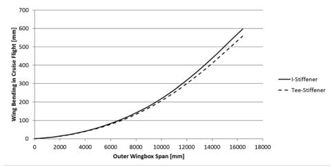
Figure 9: Comparison of Wing Bending in Cruise Flight
