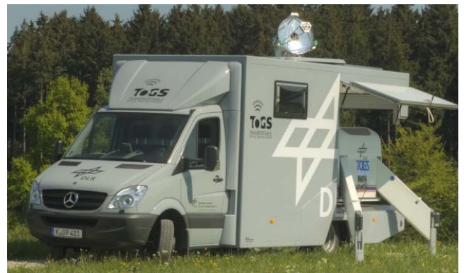
Figure 4: Transportable Optical Ground Station (TOGS)
