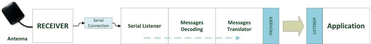
Figure 6.4: GNSS receiver interfacing
