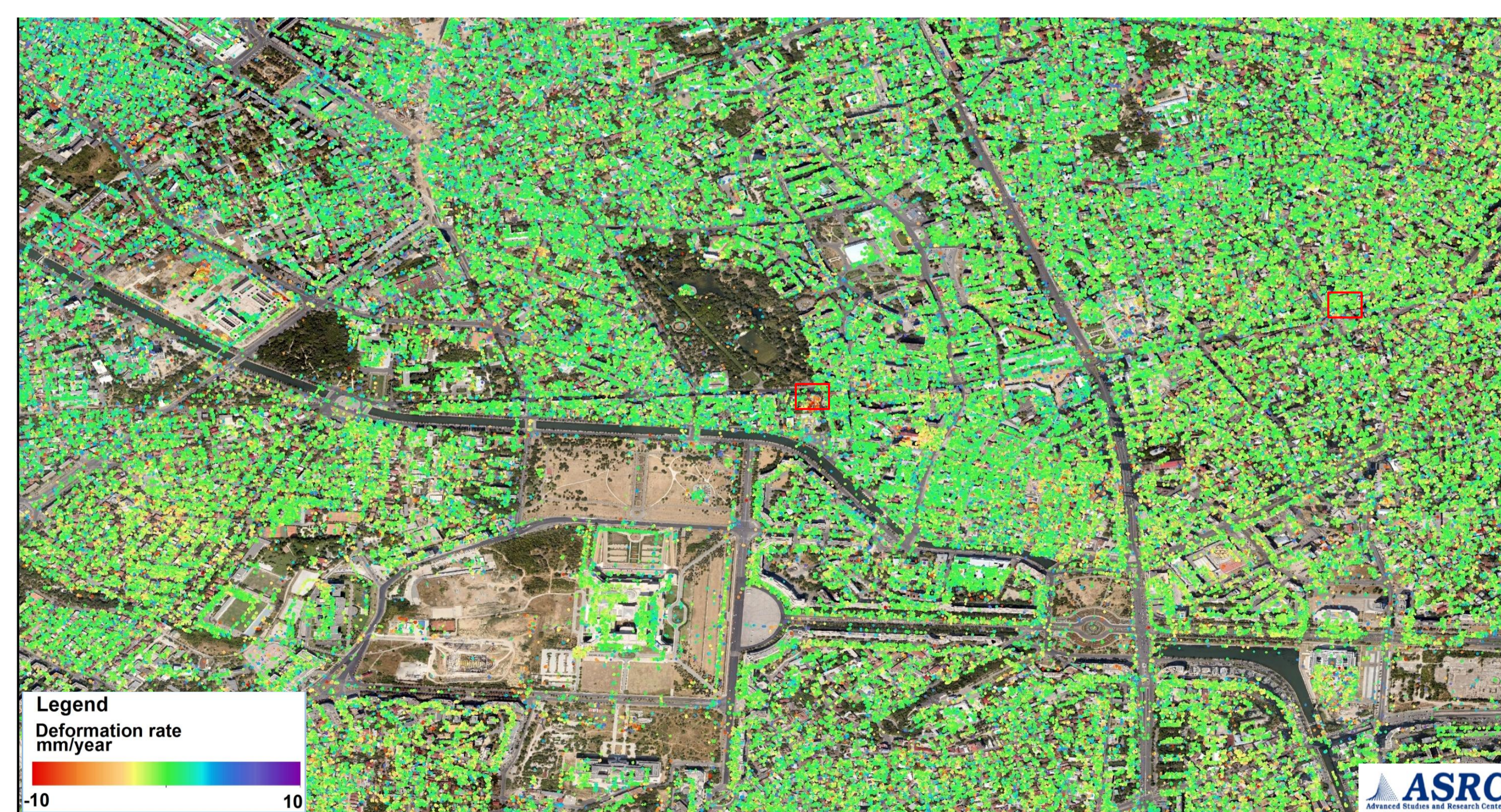
Fig. 4 Zoom-in view of the PSI deformation map on the central part of Bucharest; local subsidence and uplift areas may be identified, but also stable ones. Two examples are given in Figures 5 and 6.
