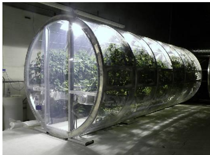
Figure 4-2: Deployed Configuration of the LGH during a test period [59]
