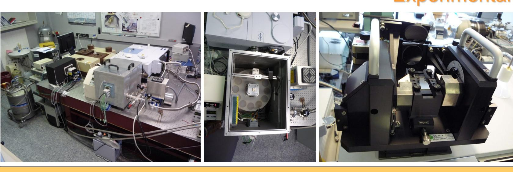
We present here new measurements on sulfates, carbonates, and phyllosilicates in various grain size ranges. The setup was configured to simulate the thermal history of surface minerals on the asteroid 2008 EV5 during its revolution around the Sun. This asteroid is the scientific target of the ESA Marco Polo-R mission.
