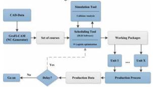
Figure 3: CAD/CAM-Chain
