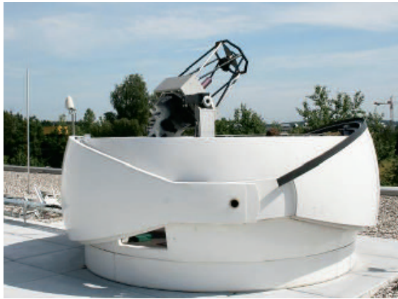
Fig.2 Image of receiver telescope in June 2009, hosted by an astronomical clamshell dome (left) and Instrument setup in the 2009 campaign (right). The beam is guided to the tracking camera, receiver front-end and measurement instruments [5]
