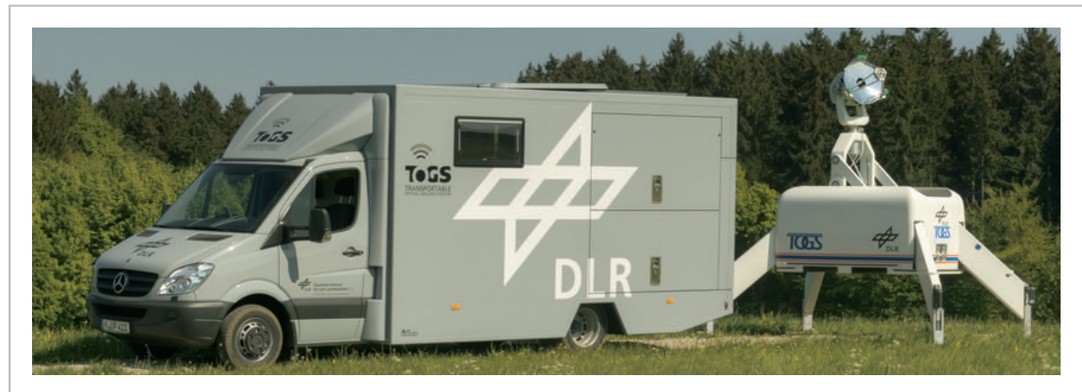
Fig.9 Transportable Optical Ground Station of DLR for Satellite- and Aircraft-Downlinks, with transport vehicle
