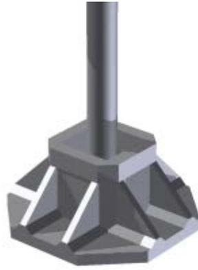
**Fig. 5. Prefabricated concrete ground-anchor foundation**
