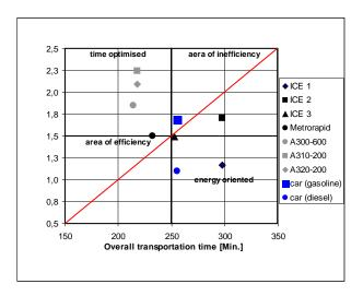
Fig. 11: Transportation efficiency on the route Schwabing – Munich – Frankfurt / Main
