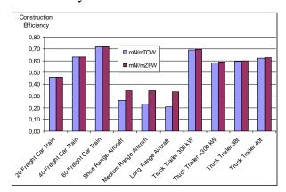
Fig. 7: Construction Efficiencies  $\eta_K$  of Different Cargo Transportation Systems
