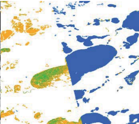
Figure 7: WAM derived the strong amplitude threshold (green), with the weaker amplitude threshold (orange) and the coherence threshold (blue)
