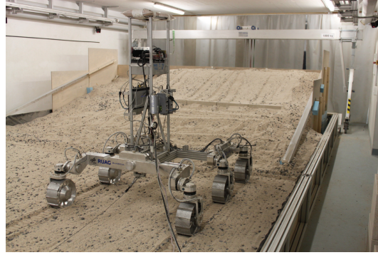
FIGURE 17: ExoMars Rover in the testbed.
