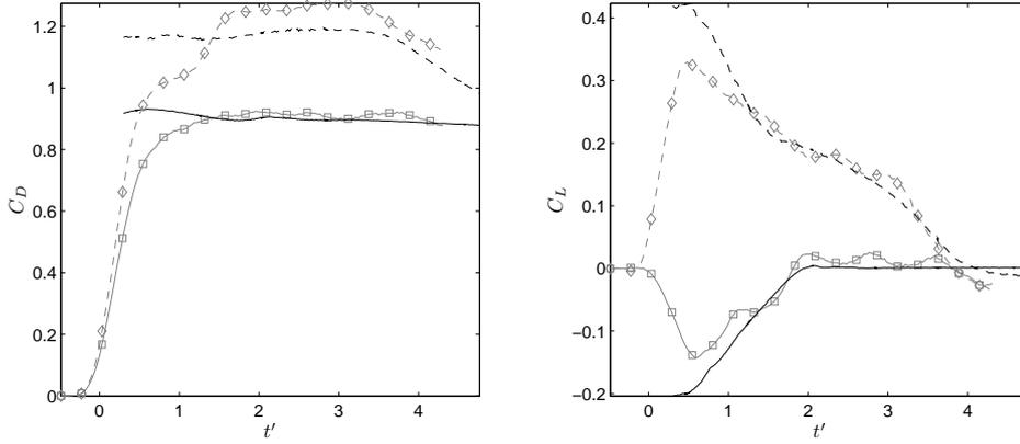
FIGURE 12. Comparison of experimental and computational force coefficients for  $r_2/r_1=0.5$  and  $\theta_0=-0.1^\circ$ :  $\square$ —, experimental primary sphere; —, computational primary sphere;  $\diamond$ —, experimental secondary sphere; ---, computational secondary sphere. The normalised variables are  $t' = \sqrt{\rho_a/\rho_m}tV/r_1$ ,  $C_D = 8a_x r/(3\rho_a V^2)$  and  $C_L = 8a_y r/(3\rho_a V^2)$ .
