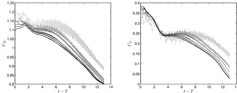
FIGURE 6. Time-resolved secondary force coefficients calculated in the six verification computations described in table 1, with the lightest to darkest curves corresponding to simulations 1 through 6.
