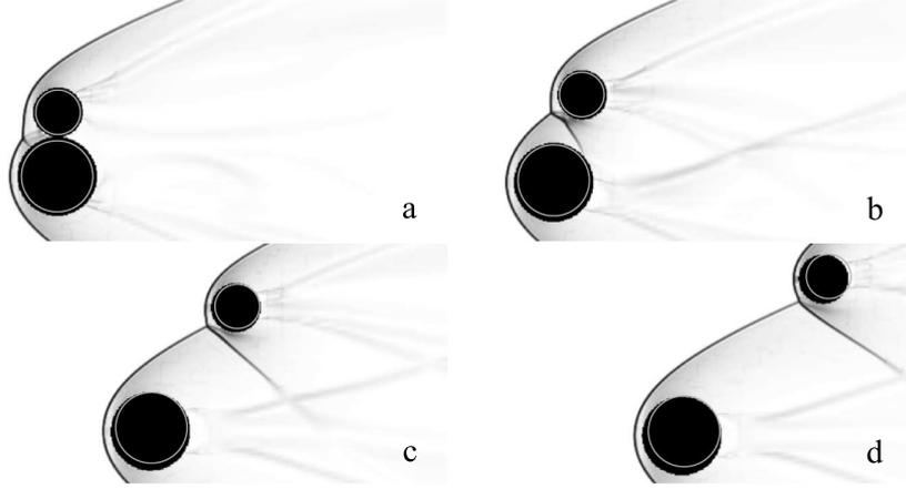
FIGURE 11. Computational Schlieren images for  $r_2/r_1=0.625$ ,  $\theta_0=-0.7^\circ$ , with equivalent experimental sphere positions (corrected for gravity) overlaid; the experimental radii are reduced by 10% for clarity. Images a, b and d correspond to the experimental images of figure 9c.
