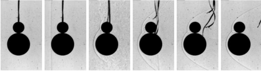
FIGURE 4. Sequence of images showing the start-up of the flow and the detachment of the threads from the spheres, at times (defined from the arrival of the initial shock):  $-0.08$ ,  $0$ ,  $0.54$ ,  $0.77$ ,  $1.00$ , and  $1.23$  ms.
