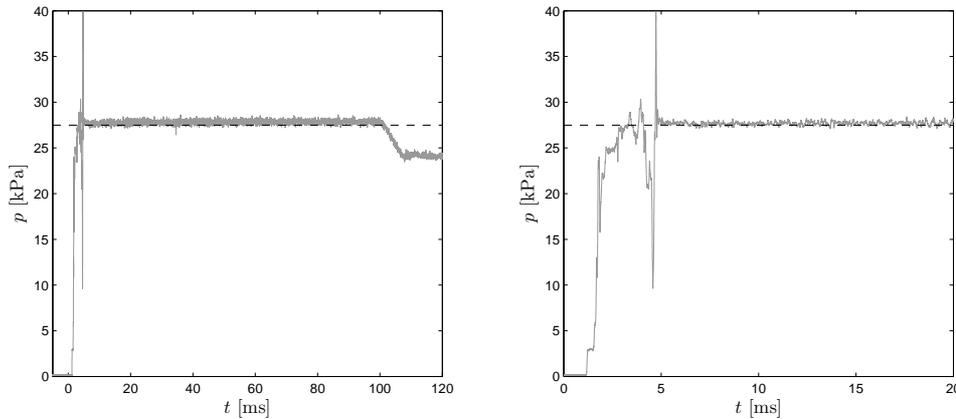
FIGURE 3. A sample Pitot pressure trace of the test-section flow: (left) showing the complete steady flow time of the tunnel; (right) showing the typical test duration employed in the present experiments. The dashed line in both plots indicates the theoretical Pitot pressure derived from the fill conditions.
