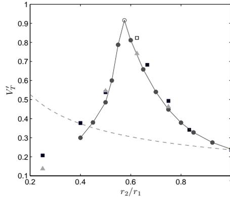
FIGURE 15. Normalised secondary separation velocities versus the radius ratio for initial axial alignment of the sphere centres:  $\square$ , experimental results;  $\triangle$ , refined computational result with identical initial alignment angles to experiments;  $\circ$ , coarse computational result with  $\theta_0=0$ ; ---, prediction of Passey & Melosh (1980). Open points indicate extrapolated values.
