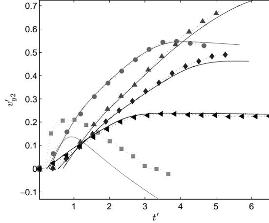
FIGURE 13. Normalised secondary lateral velocities as functions of the non-dimensional time in experiments (symbols) and numerical simulations (lines only in matching shades):  $\square$ ,  $r_2/r_1=0.25$ ;  $\circ$ ,  $r_2/r_1=0.5$ ;  $\triangle$ ,  $r_2/r_1=0.625$ ;  $\diamond$ ,  $r_2/r_1=0.75$ ;  $\blacktriangleleft$ ,  $r_2/r_1=1$ .
