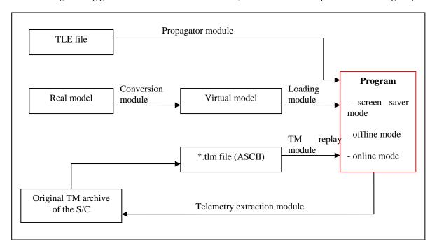
Figure 2: General architecture of SatelliteSim tool
