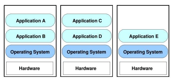
Figure 1. Current control room setup. Each workstation with locally installed O/S is used for one well-defined type of task.
