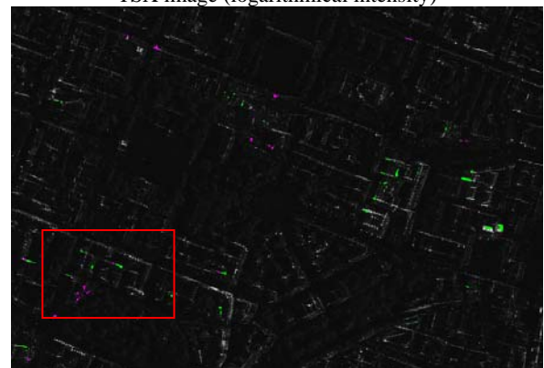
Figure 5. Change Results by analysis of shadow (cyan) and ground areas (magenta), overlaid on scaled TSX image
