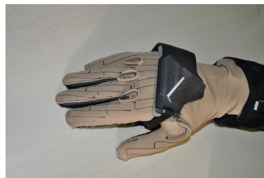
Figure 1.2: Cyberglove together with the handle of the HMI
