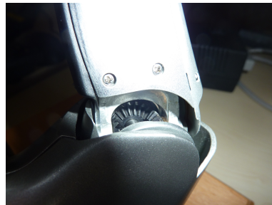
Figure 1.5: Bevel gears at the base joint
