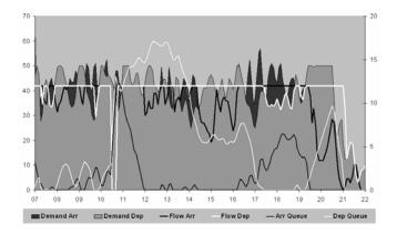
Figure 11. Flow trends (as Fig.7) – for case of runway system ihibition for 15 minutes (10:30–10:45) (non optimized reference).
