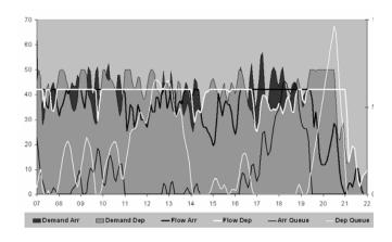
Figure 7. Flow trends of arrivals and departures relative to respective demands for simulated not optimized operations (left axis), together with resulting holding queues (right axis).
