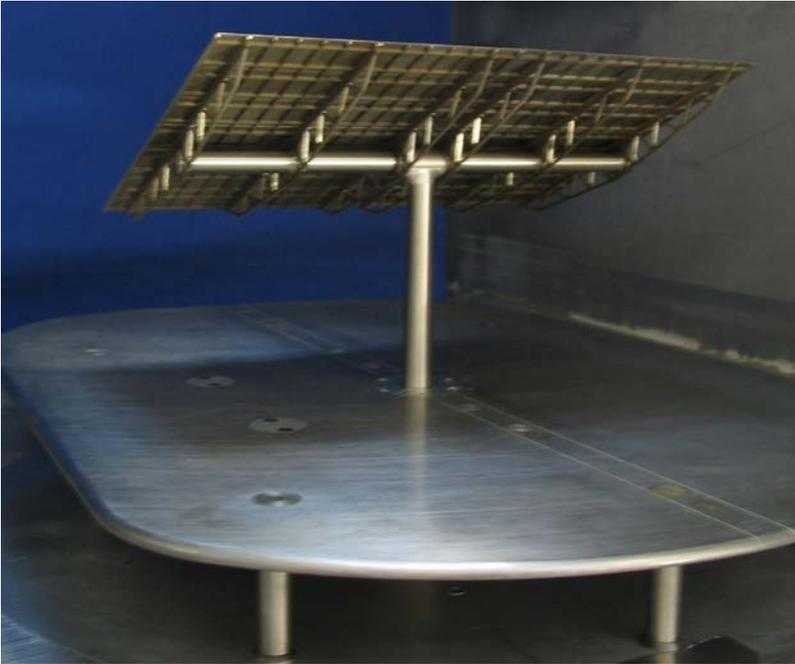
**Figure 6: Heliostat model in HDG, scale 1:50**
