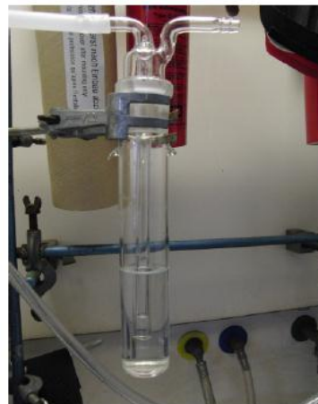
(a) The washing flask before carbon corrosion experiment for GDL 25BC Std.
