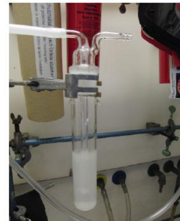
(b) The washing flask after carbon corrosion experiment for GDL 25BC Std.
