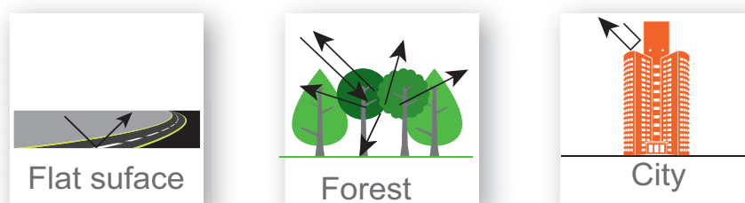
Figure 2.4: Examples of different levels of backscattering. Flat surface will appear as dark area in a SAR image. Forest areas, reflects medium backscattering. Backscattering over cities will appear as bright area in a SAR image.
