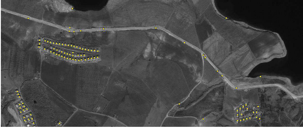
Fig. 3. Building detection results using steerable filters on a sample large Ikonos test image.
