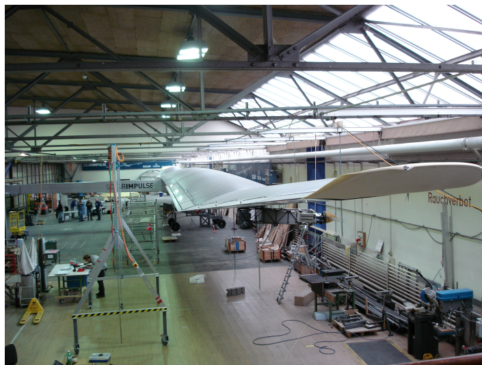
Figure 6: GVT on fully assembled Solar Impulse
