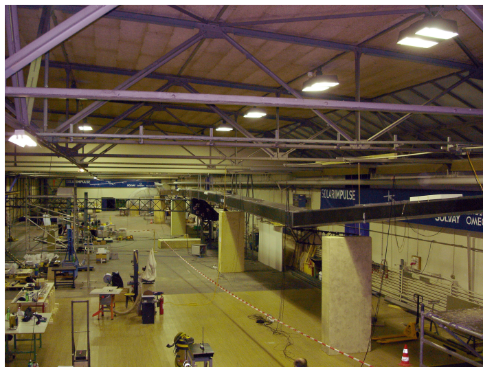
Figure 3: GVT on 1 st assembly of the primary structure of Solar Impulse
