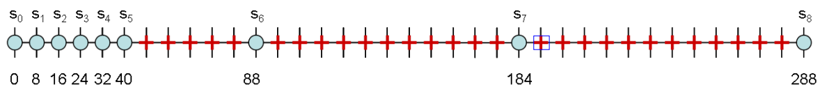
Figure 6: Tomographic constellation of 9 images ( s_0, \dots, s_8 ) at P-band. Acquired track (blue circles) and virtual tracks (red crosses). The baselines are indicated in meters beneath the circles.
