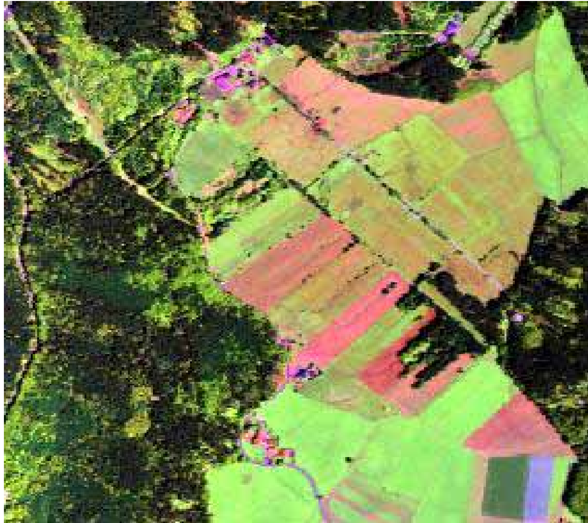
Hyperspectral data with 128 spectral channels (RGB - 79 / 41 / 9)
