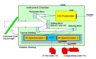
Figure 7: Instrument chamber schematics
