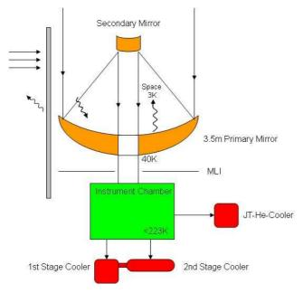
Figure 6: Telescope configuration
